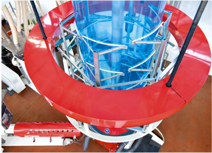
Fig. 2. The Optimex, previously only available as a 3-layer system, is now also offered as a 5-layer system
