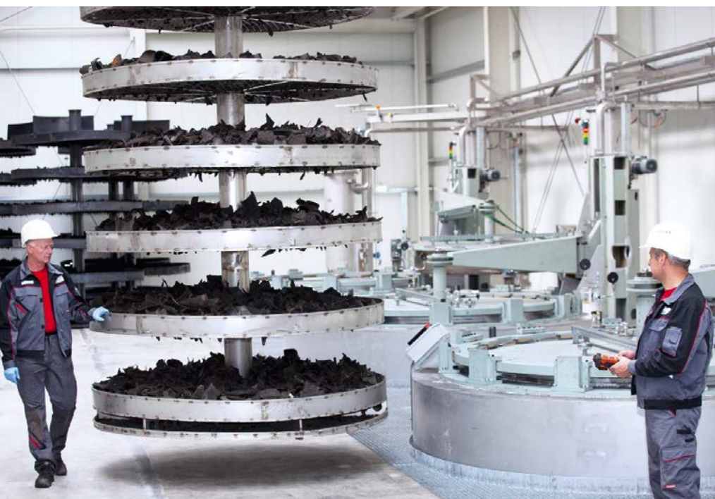
Production of recovered carbon black at the cct plant. The material from used tires comes roughly shredded and is conveyed to the pyrolysis reactors (© cct)
