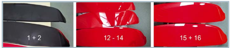
Fig. 6. A color change from black to red with a non-flow-optimized hot runner requires 16 cycles with the Flexflow technology (some of which are shown above), but without this support, 35 cycles (© HRSflow)
