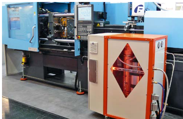
Fig. 8. The heating unit (foreground) feeds CO 2 which has evaporated in the cooling phase back into the process to heat the mold in the next cycle (figure: gwk)
