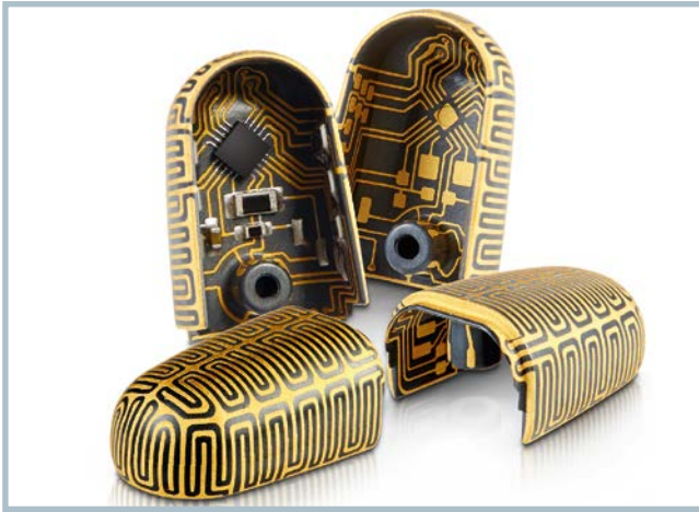
Fig. 3. Finger of a robot hand as an MID component. The laser process not only creates the 3-D structures, but also makes the interconnects (figure: LaserMicronics)
