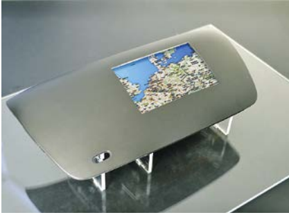
Fig. 6. Touch-sensitive panel demonstration part. The film printed with transparent conductor tracks is back-molded in the IML process – the transparent plastic panel in the figure on the right permits a view of the interior (figure: Display Solution)
