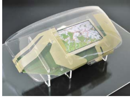
Fig. 6. Touch-sensitive panel demonstration part. The film printed with transparent conductor tracks is back-molded in the IML process – the transparent plastic panel in the figure on the right permits a view of the interior (figure: Display Solution)
