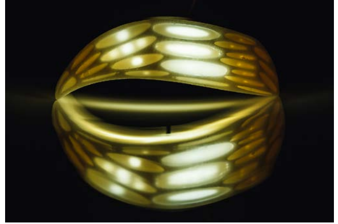
Fig. 7. LED and optical waveguide integration with PFLM. By interrupting the layer build-up and placing an insert, the various components can be integrated without an assembly step (figure: Fraunhofer IPA, Covestro)
