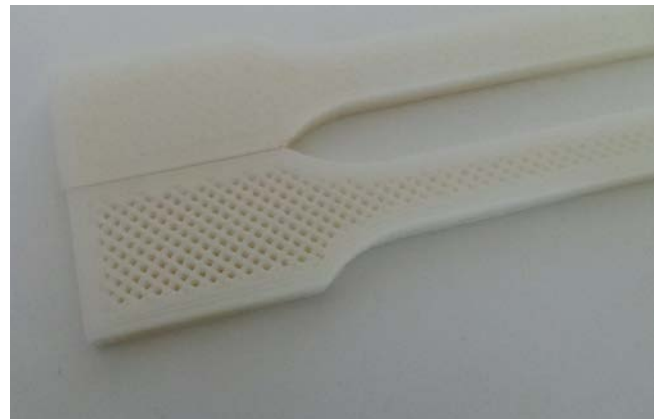
Fig. 5. Filling strategy with 45° hatching: depending on the design, it allows solid filling or a hollow structure to be produced (figure: Fraunhofer IPA)
