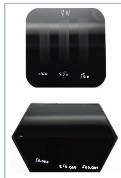
Fig. 3. Comparison of the abrasion resistance (Crockmeter with wool felt 9N) of test parts made from PMMA (above) and parts produced by the CoverForm process (below)
