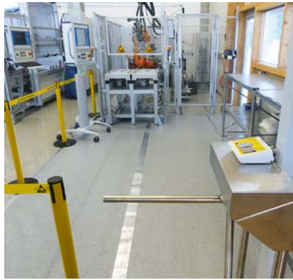
Certified protection zone for ESD-compliant foam gasketing, gluing, and potting at Sonderhoff PSA in Dornbirn (left). The contract manufacturer specializes mainly in micro gasketing and micro potting small components for the IT/electronics industry and medical technology
