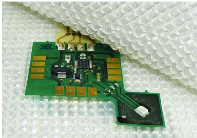
**Fig. 2.** The electronic components of the sensor network are inserted between two layers of hybrid yarn-based GF/PP multi-layer knitted fabric (© ILK, TU Dresden)
