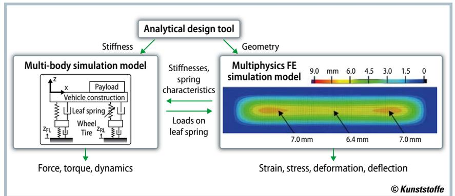
**Fig. 4.** Static and dynamic behavior of leaf spring and vehicle were simulated with the help of various calculating tools (source: ILK, TU Dresden)
