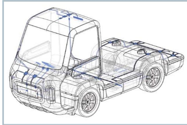
**Fig. 3.** Overview of the trans-component, composite-integrated sensor network of the demonstrator vehicle (© ILK, TU Dresden)
