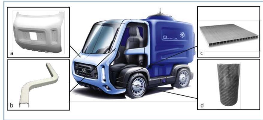
**Fig. 1.** Highly integrated structural components in the driver's cabin: (a) complex-shaped front shell made of GF/PP multi-layer knitted fabric, (b) vehicle column made of near-net shape knitted preform, (c) textile composite spacer structures, and (d) bonded joint (© ILK, TU Dresden)
