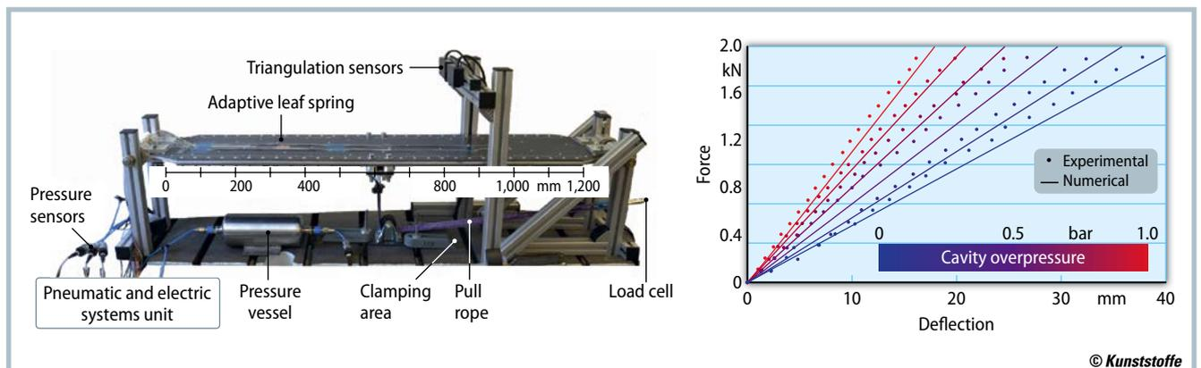
**Fig. 5.** Experimental test setup with installed leaf spring (left), whereby spring characteristics were determined experimentally and by means of a calibrated finite element model (right) (source: ILK, TU Dresden)
