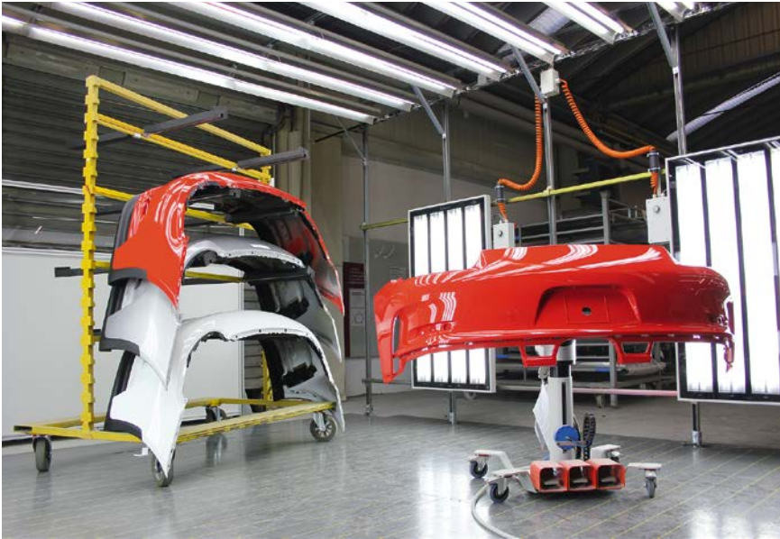
Fig. 2. View of rear apron production in Hörsching, Austria. The components are not only produced here but also receive a class A paint finish. The site specializes in short-run production of automotive exterior parts (© Polytec Group)
