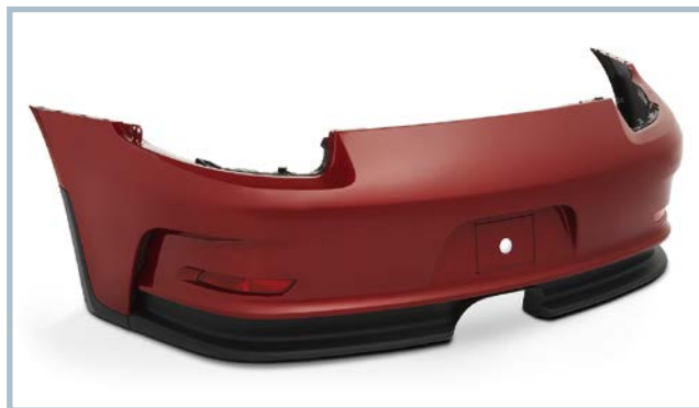
Fig. 1. The design freedom offered by the polyurethane system is not only exploited to advantage in the size and complex shape of the rear apron but also permits a high degree of functional integration (© Polytec Group)
