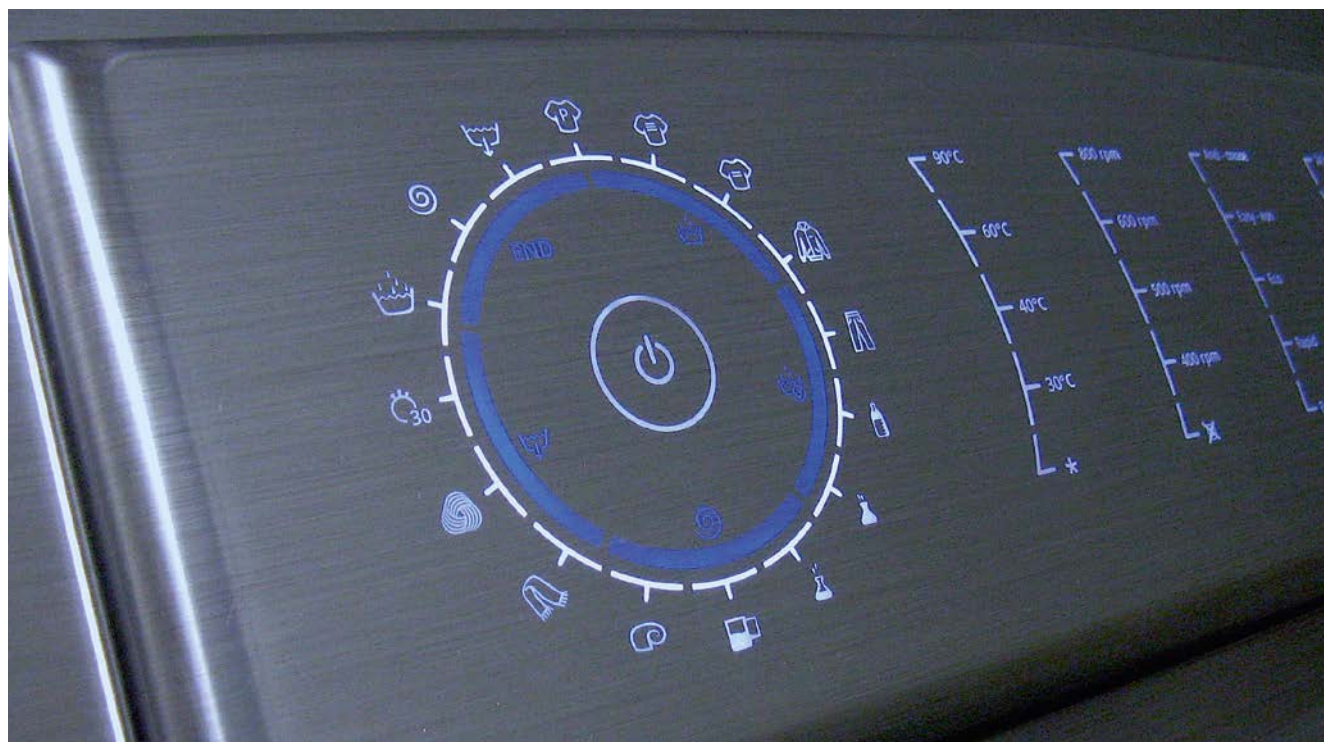
The current stage of development of Multiskin composite films allows the production of three-dimensionally shaped user interfaces, for example with profile areas for finger guidance (© plastic electronic)
