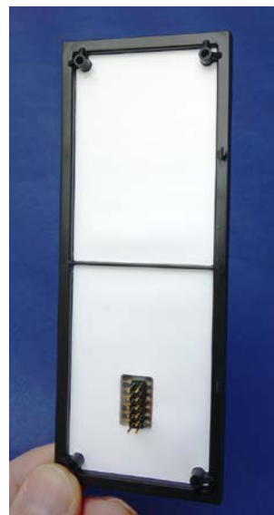
Fig. 4. One way to reduce the shrinkage effects on the composite film is by in-molding with a frame structure, which also acts as a carrier for the mechanical interfaces to the partner components; shown here with the example of a 2.2mm laminated composite panel with integrated lighting system and 12-pin connector (© Schöfer GmbH)
