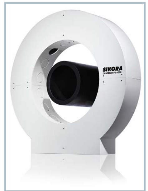
Fig. 1. Millimeter wave measuring technology: the system has a clear span of 600 mm and determines diameter, ovality, wall thicknesses and sagging of large tubes. By means of two transceivers (one transceiver is positioned top left in the measuring system) all measuring values can simultaneously be measured at four points of the circumference (© Sikora)
