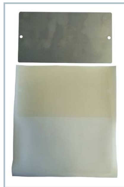
Fig. 5. Reproduction of discoloration: testing a painted surface containing several light stabilizers and antioxidants as well as silver contamination after solar simulation in accordance with VDA 230-219; the top area of the sample was covered with a metal sheet (above) (© Daimler)
