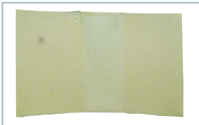
Fig. 4. Metals catalyze the discoloration: selective discoloration of paints due to metal agglomeration after aging in artificial light at high temperature (discolored areas left and right were covered with a metal sheet)
