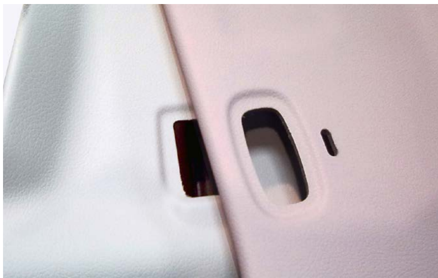
Automobile C pillar laminated to thermoforming film: in the dark, the component underwent pink discoloration (front right). On exposure to light, the discoloration was reversed (original, back left) (© Daimler)
