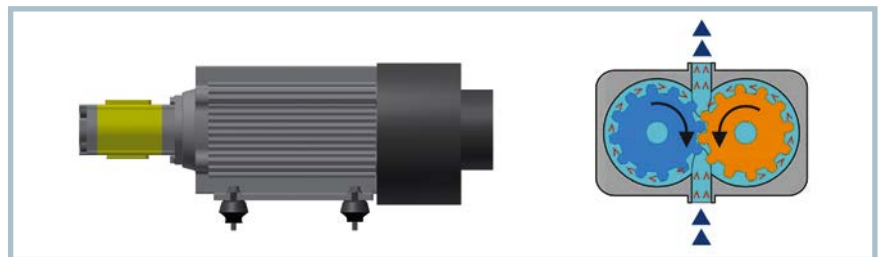
Fig. 5. Servo drive with fixed displacement pump: When no pump capacity is required, the servo motor switches off (© Dr. Boy)
