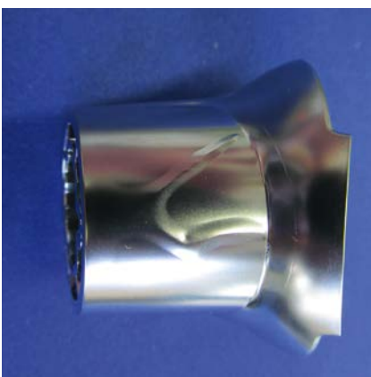
Fig. 3. Delamination as possible failure and surface defect caused by climate change tests (© BIA)
