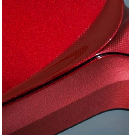
Fig. 2. The gloss levels of the effect lacquer system range from high gloss to matt; surfaces can be smooth, textured or feature a soft feel (© Covestro)
