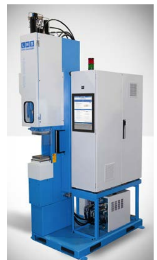
Fig. 9. The "Micro Class" micro injection molding machine has a footprint of just approx. 1 m 2
