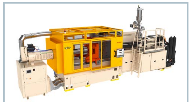
Fig. 7. The new HyCap 4 produces bottle closures while consuming 40% less energy (© Husky)
