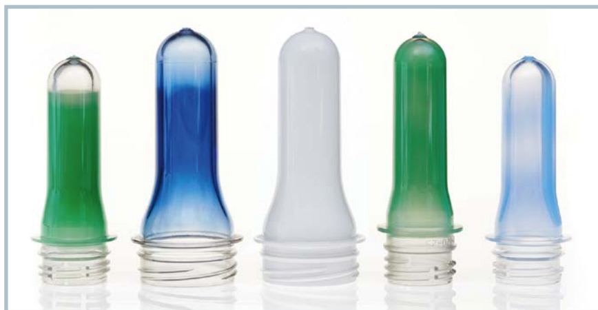
Fig. 3. Preforms for bottles with pigmented barrier layers for different applications. Containers with thick-walled bases do not require a barrier around the gate point (© Husky)
