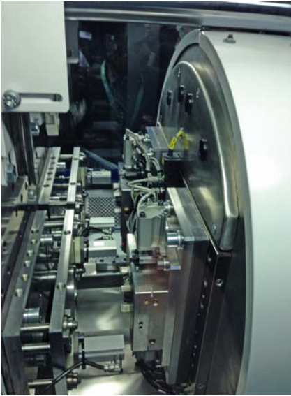
Fig. 6. Rotary table of the micro injection molding machine with two independent injection molds for preform and finished part. The blue component is electrically conductive (© Wittmann Battenfeld)
