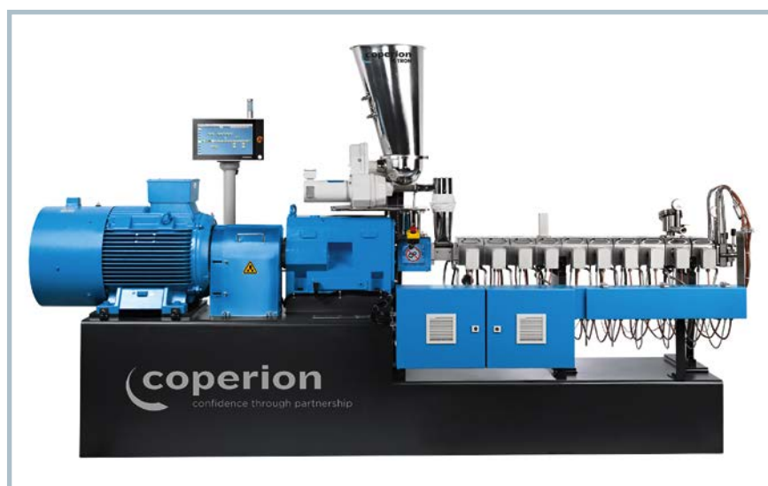
Fig. 1. Further development: the STS Mc 11 compounding system features improved operational reliability and ease of use (© Coperion)
