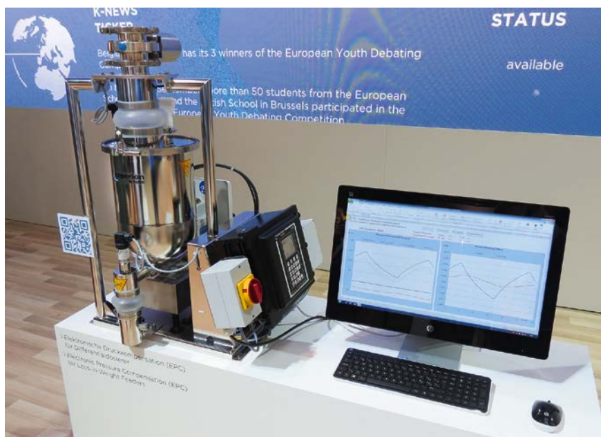
Fig. 8. Differential dosing feeder: exact dosing by means of electronic pressure compensation
