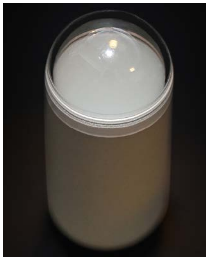
Fig. 5. The PC material Makrolon used in the casing of a capsule endoscope is biocompatible and, thanks to its good moldability, makes a large camera opening angle possible
