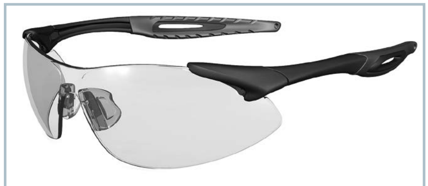
Fig. 7. The lenses in safety goggles from MCR Safety are made of the impact-resistant PC material Makrolon 3207 of Covestro. They are lightweight, hard, and feature high optical quality and impact resistance in addition to good UV protection (© MCR Safety)
