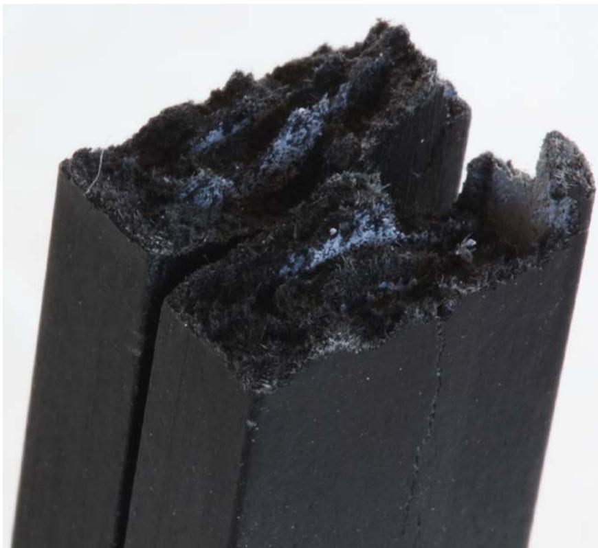
The fracture surface of a 4 mm specimen of glass-fiber-reinforced polyamide 66 with a longitudinal crack (© IKT)
