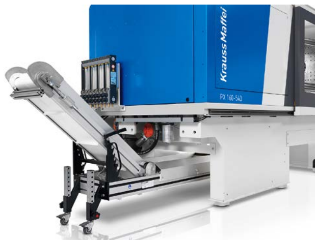
Fig. 1. The machine bed of the PX offers space for the easy integration of conveyor belts (© KraussMaffei)
