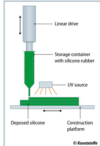
**Fig. 2.** Principle of the printing process: Silicone is extruded from the storage container and deposited in lines on a construction platform. A UV source donates the required cross-linking energy (source: IKV)
