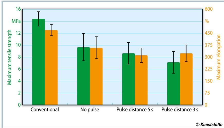
**Fig. 3.** Comparison of the maximum tensile stress and elongation of conventional and additive manufactured specimen under variation of pulse distance (source: IKV)
