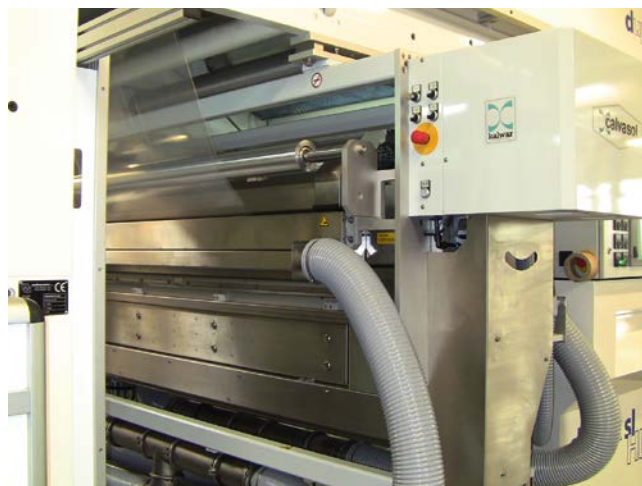
Fig. 3. The Calvasol system can be integrated directly into the lamination process with no negative influence on the lamination adhesive (© kalwar)
