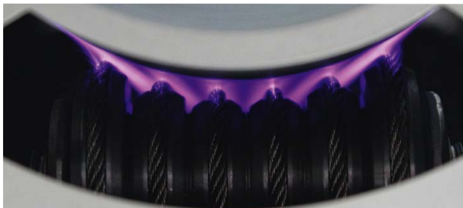
Fig. 2. The aerosols are applied to the film from below. This has the benefit that the functional molecules can be anchored in a very thin and even layer (© kalwar)
