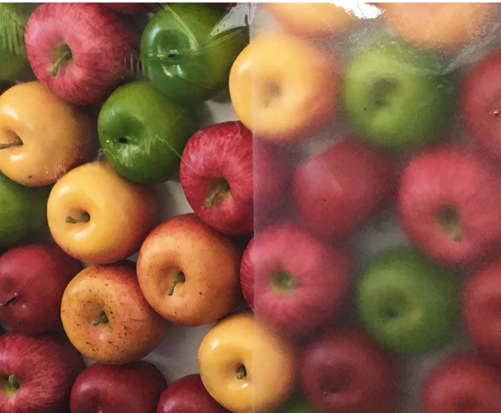
A clear view: Preventing the fogging of food packaging film is important. Corresponding functionalizing additives in aerosol form can be applied in a very thin layer to accomplish this
