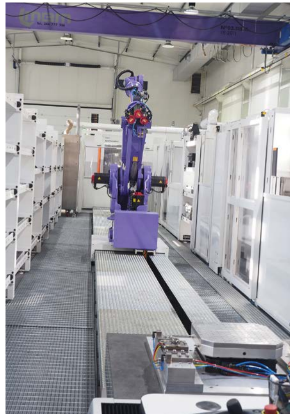
Fig. 1. Fully automatic manufacturing cell with programmed mold changing unit at Moldes RP (© Hanser / C. Doriat)
