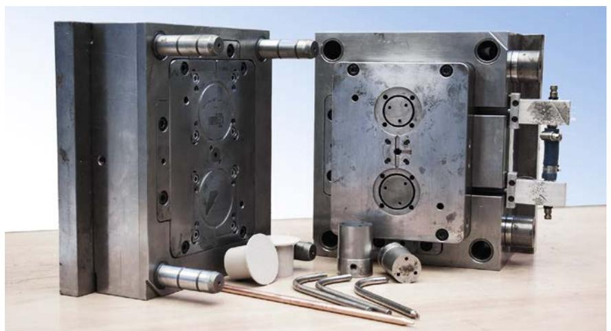
**Fig. 5.** No-cool mold for a cap application; the heat pipes and removed core inserts are shown in the foreground (© Bielefeld University of Applied Sciences)
