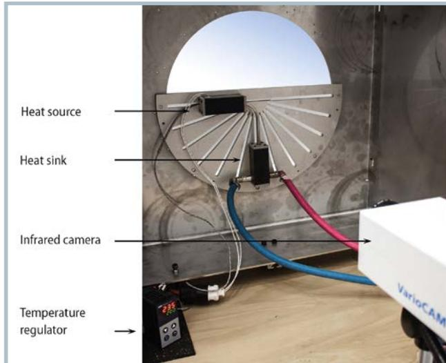
**Fig. 6.** Test rig for determining heat pipe characteristic maps. The temperatures at the two copper blocks are read with an infrared camera
