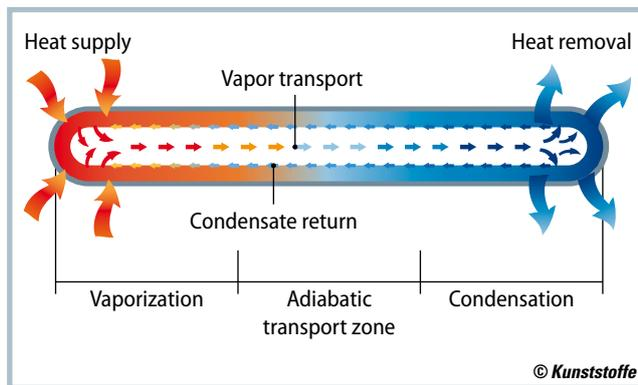
**Fig. 2.** Heat pipes exploit the temperature difference between heat source and heat sink (source: Bielefeld University of Applied Sciences)
