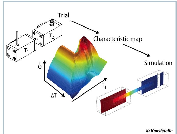
**Fig. 7.** The characteristic map of a heat pipe shows the transferable heat capacity as a function of local temperatures (source: Bielefeld University
