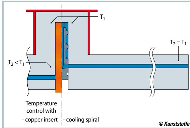
**Fig. 1.** Conventional temperature control of cores is based on the use of heat-conducting inserts or the flow of liquid media (source: Bielefeld University of Applied Sciences)
