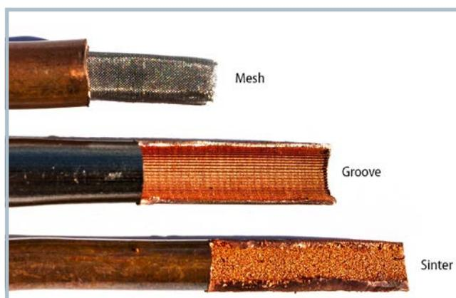
**Fig. 3.** The capillary effect can be generated by different internal structures in the heat pipes (© Bielefeld University of Applied Sciences)
