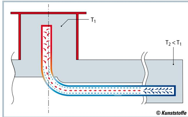
**Fig. 4.** Controlling the temperature of a core with a heat pipe (source: Bielefeld University of Applied Sciences)
