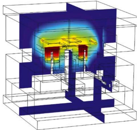
Heat pipes support rapid heat exchange. It is not absolutely essential to remove all the heat of the melt from the mold. It is also possible to define climatic zones in areas remote from cavities, into which some of the heat is directed (© Bielefeld University of Applied Sciences)
