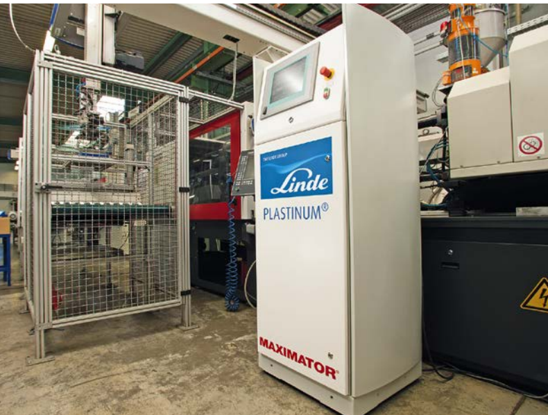
Fig. 6. The pressure control module (Linde) has to respond quickly and keep the counter-pressure constant to the end of the flow path by releasing gas as the melt flows in (© Linde)
