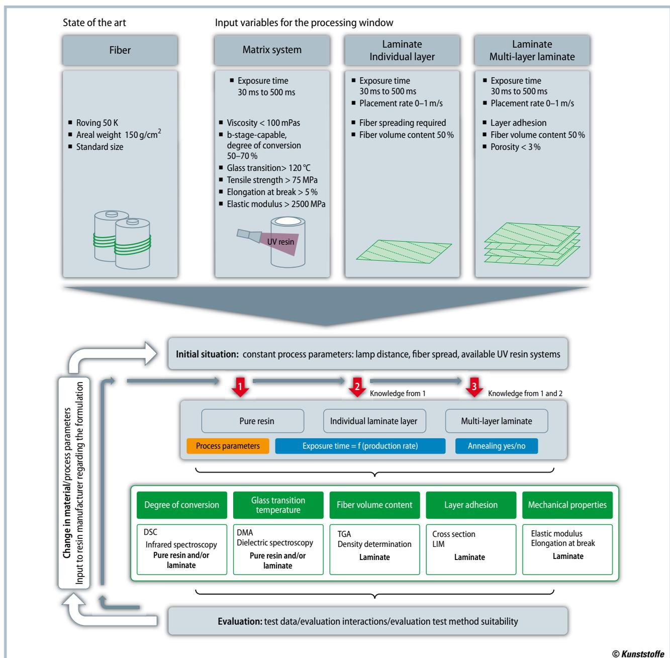
**Fig. 4.** Material requirements and selection system to meet the necessary process criteria (source: R. Hofmann)
