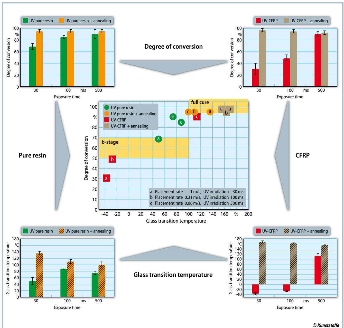
Fig. 6. Graphic representation of the different pure resin and laminate results for placement speeds of 1 m/s, 0.31 m/s and 0.06 m/s. The middle graph shows the degree of conversion as a function of exposure time (a, b, c) and glass transition temperature. The target states for the placed laminate layers (b-stage) and final CFRP laminate (full cure) are indicated in yellow (source: R. Hofmann)
