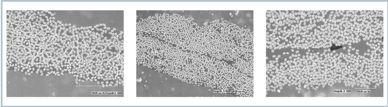
**Fig. 7.** Light micrographs of a UV-cured individual laminate layer, a multi-layer laminate (b-stage/b-stage) and a multi-layer laminate (b-stage/full cure). The samples were produced without a press (from left to right) (© R. Hofmann)
