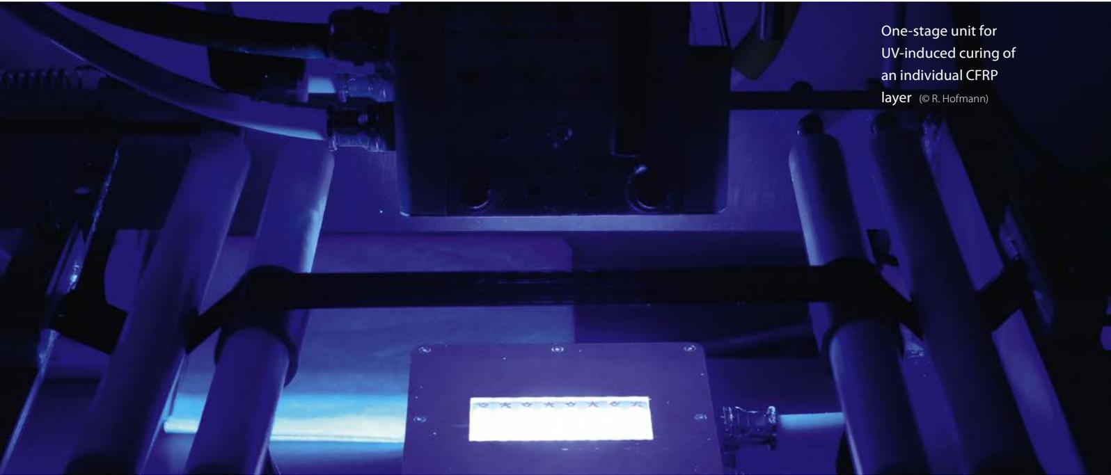
One-stage unit for UV-induced curing of an individual CFRP layer © R. Hofmann
