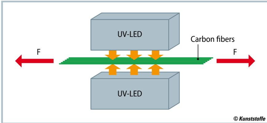
Fig. 5. Static test installation for the production of single laminate layers using UV curing
