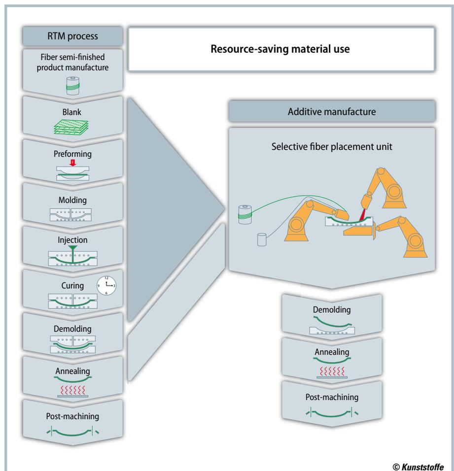
Fig. 1. Comparison between the CFRP manufacturing processes of resin transfer molding (RTM) and selective fiber placement: from the roving directly to the component (source: R. Hofmann)
