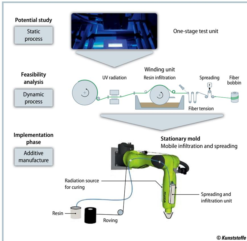
**Fig. 2.** Test chain from the static process over the dynamic process to the pilot-scale additive manufacture (source: R. Hofmann)
