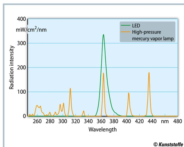
**Fig. 3.** Comparison between the wavelengths emitted by representative mercury vapor and UV-LED lamps (source: R. Hofmann)
