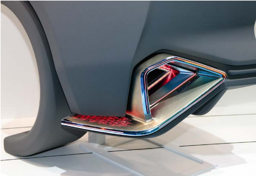
Fig. 2. Due to the PC HT+ABS blends, LEDs can be integrated into the exhaust trim to make the part more attractive (© Covestro)
