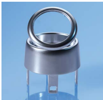
Fig. 1. Optically difficult to distinguish: Chrome lacquer (top), galvanized coat (bottom) (© Kunststoff Helmbrechts)
