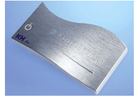
Fig. 5. The recipe for cool haptics with “Cool-Brush”: A laser-structured mold and thermally conducting plastic plus chrome lacquer
