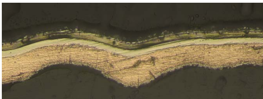
Fig. 4. Microscopic image (magnified 10,000 times) of a cut through the layer composition of a brushed surface subsequent to electroplating. All layers are uniformly intact and not damaged by subsequent laser treatment (© BIA)
