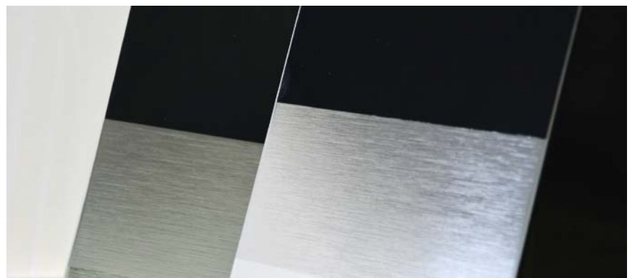
Fig. 2. The new process gives the chrome layer both the look and the feel of a brushed surface. It creates a high-quality overall impression and enables a selective distinction to unstructured areas (at the top of the picture) (© BIA)
