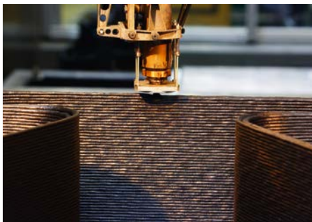
A new family of high-performance Thermocomp AM compounds addresses the unique requirements of large format additive manufacturing (LFAM) (© Sabic)
