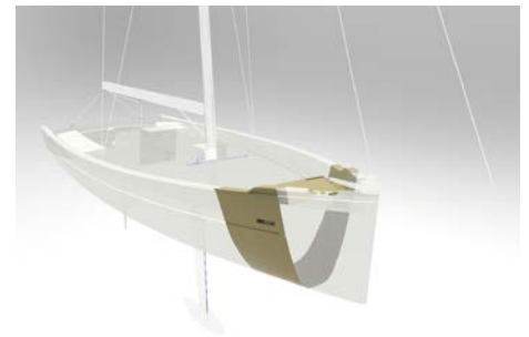
Two materials from the new Thermocomp AM portfolio were selected for a yacht hull from Livrea Yachts – a carbon-fiber-reinforced PPE compound for the hull's outer layer, and carbon-fiber-reinforced PEI for the inner lattice support structure (© Sabic)
