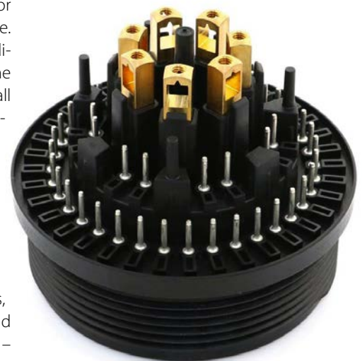
Fig. 6. 57 metal contacts are positioned precisely in the mold before overmolding
