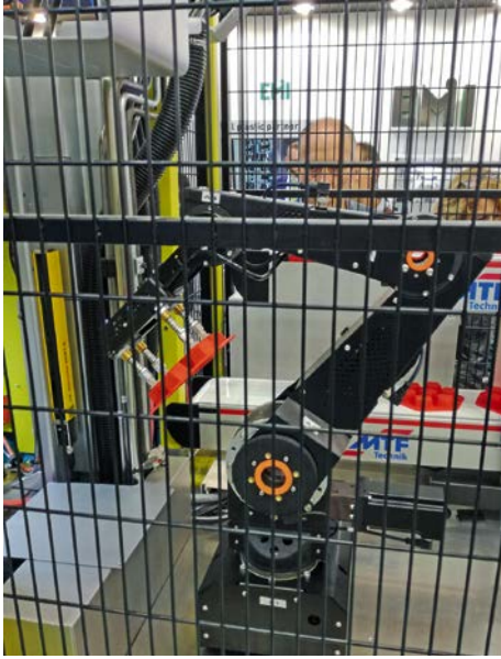
Fig. 3. The four-axis robot from Igus is an inexpensive handling solution for many tasks (© Hanser/ C. Doriat)
