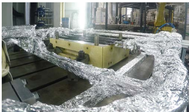
Fig. 3. The gripper-assisted forming process prevents the composite laminate from touching the forming dies too early © Fraunhofer ICT
