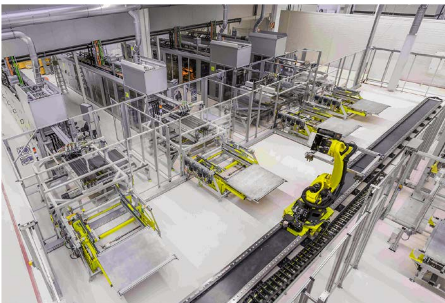
Fig. 2. View into the Voith production facility at Garching, close to Munich, Germany. There, the Audi A8 CFRP rear wall structure is processed in a fully automated manufacturing process utilizing the patented direct fiber placement technology by the Voith roving applicator (© Voith Composites)
