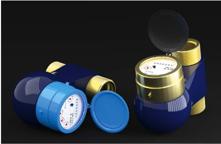
The mountings for dial indicator glasses (for a water meter in this example) have previously been made of brass and the sight glass mechanically screwed-on. Now, the brass can be replaced with plastic and the glass completely overmolded (© Pentacon)
