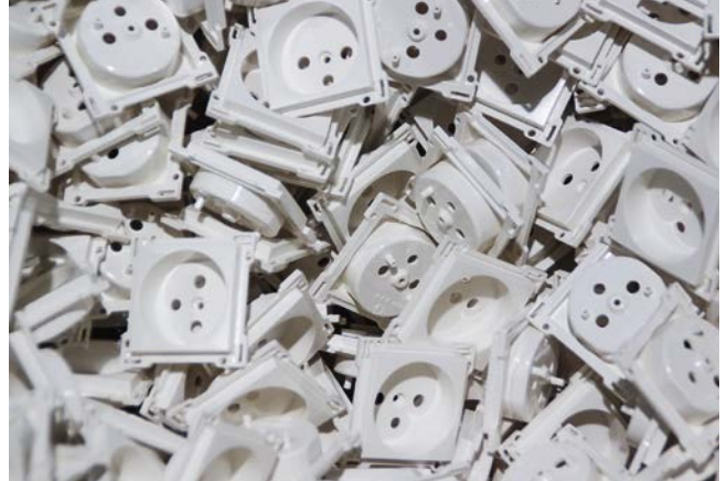
The production of the plug outlet covers is converted to an 8-cavity injection mold with electrically operated hot runner valve system
