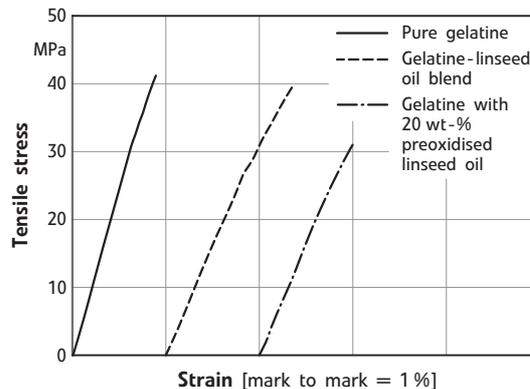
Fig. 2. Tensile stress-strain curves of pure gelatine and of gelatine blends with 20 wt-% pre-oxidised linseed oil (lecithin content 5 wt-%) (hardened at 170 °C)
