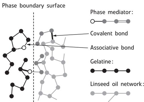
Fig. 1. Schematic representation of the phase boundary surface of gelatine and linseed oil with phase mediator
