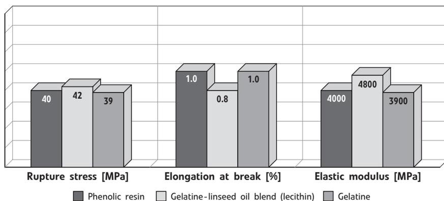
Fig. 3. Mechanical characteristics of gelatine-linseed oil blends and of phenolic resin
