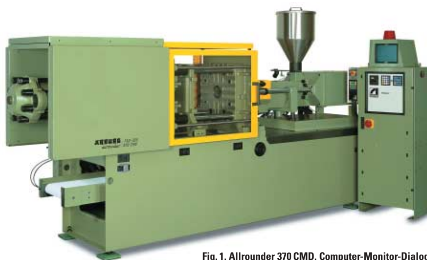
Fig. 1. Allrounder 370 CMD. Computer-Monitor-Dialog: The computer was used for control and monitoring the machine, the monitor for displaying data and functions (1983) (Photo: Arburg)
