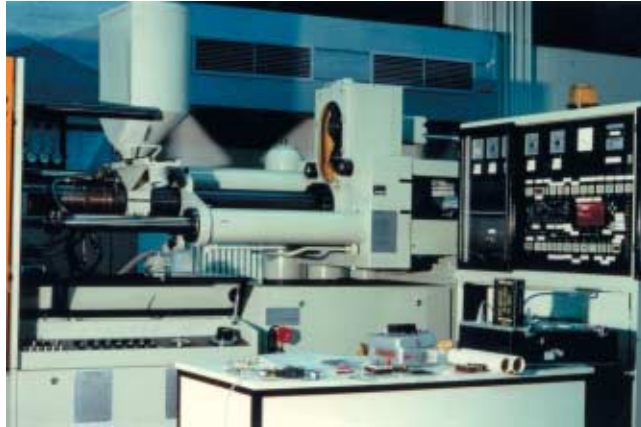
Fig. 2. Injection moulding machine with switch cabinet from the early eighties in the IKV pilot plant (Manufacturer: Battenfeld)
