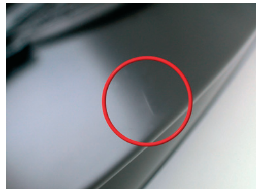
Fig. 3. Sporadically occurring crazing on the part without automatic cooling time computation
