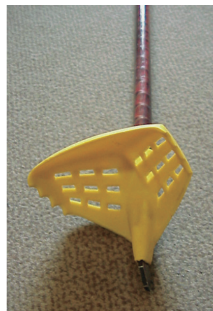
Fig. 4. The disc with integrated spike is plugged onto the lower cylindrical shaft part
