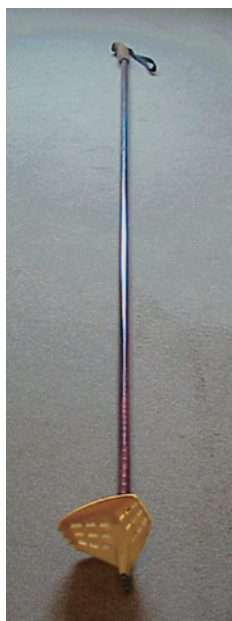
Fig. 2. Prototype of a complete GRP cross-country ski pole
