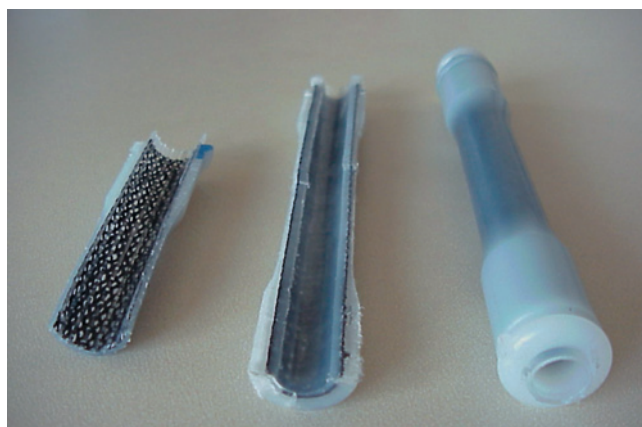
Fig. 5. Test specimen of the hybrid process for reinforced layer structures
