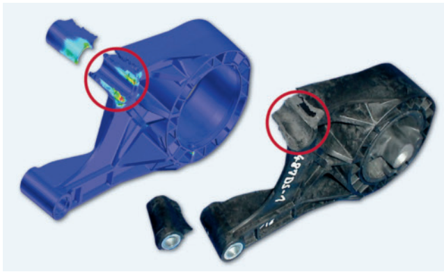
Fig. 9. Predicted fracture load: 14.4 kN; tested fracture load: 14.4 to 15.0 kN
