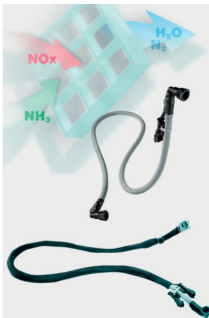
Fig. 1. EPDM hoses made from peroxide-cured EPDM survive contact with urea without hardening. The plasticizer-free formulation also prevents contamination of the catalyst (picture: ContiTech)
