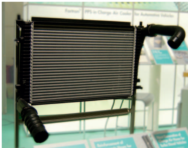
Fig. 3. For the highly stressed supercharger segment elastomer hoses reinforced with PPS multifilaments have been developed (photo: Ticona)
