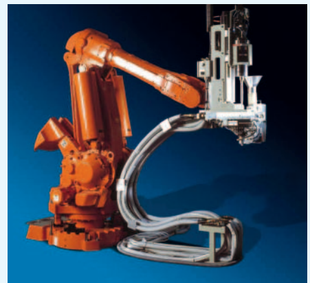
Fig. 3. Self-cleaning low-pressure mixing head (photo: Desma)
