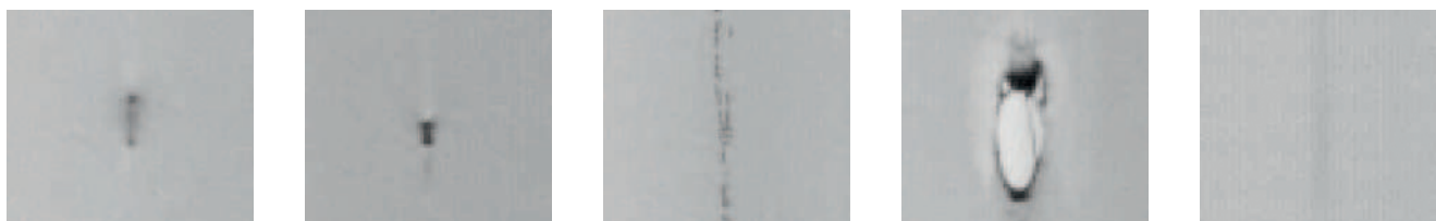
Fig. 2. Images of film defects (from left to right: speck, black spot, structure, hole, burn)
