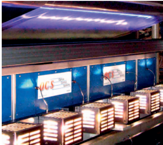
Fig. 10. Illumination concepts for detection of optical film defects
