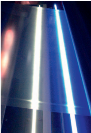
Fig. 10. Illumination concepts for detection of optical film defects
