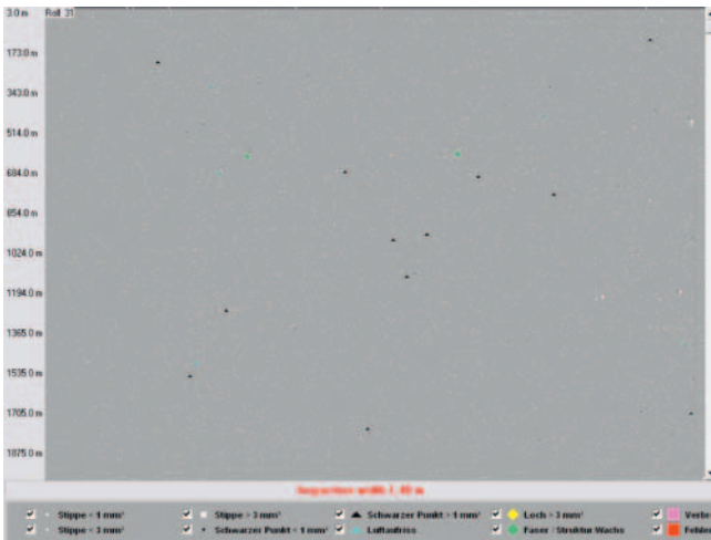
Fig. 4. Image of film surface (left), detected defects as logged (rights)
