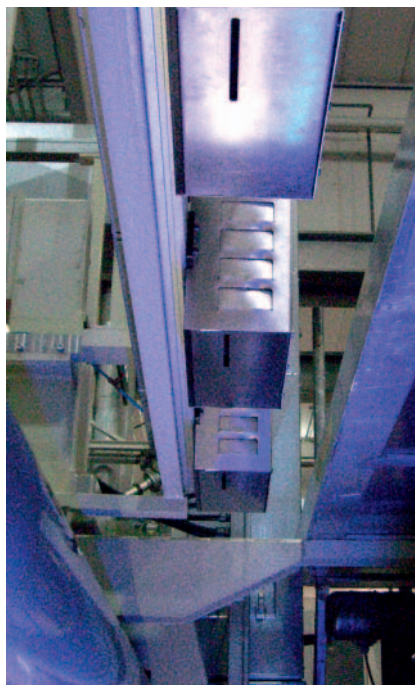
▲ Fig. 9. Examples of integration of OCS camera systems in calender lines
