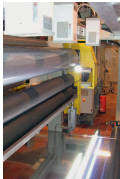
▲ Fig. 9. Examples of integration of OCS camera systems in calender lines
