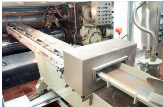
Fig. 8. Conveyor belt for supplying material to a calender line
