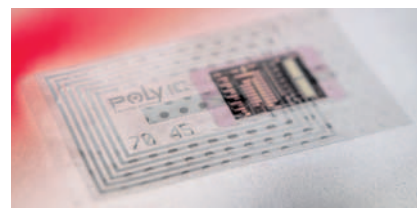
Fig. 9. First printed electronic products ‘off the reel’ (PolyID RFID tag)
