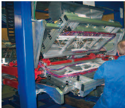
Easy and quick exchange of an IR source
