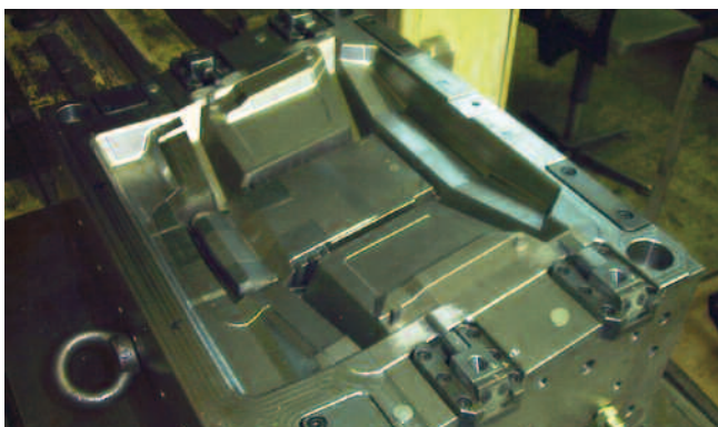
The mould for forming the seat support part during the final inspection on the touch up press (photo: Deckerform)
