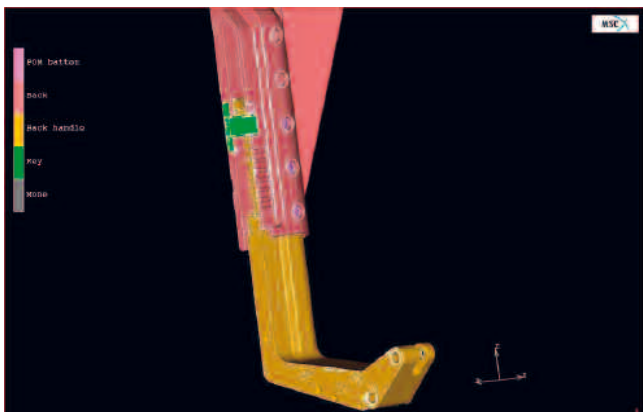
The back assembly in the FEM computation (picture: Ito Design)
