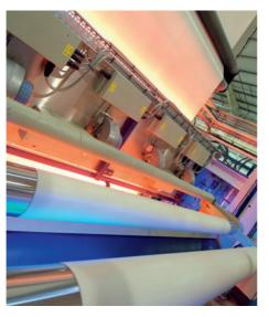
Infrared radiators quickly and reliably dry silicone coatings on plastics tissues Heat Treatment. Coated safety materials, such as those used e.g. in airbags, have to meet high quality standards. When infrared radiators are used for drying and preheating, the process can be controlled individually and the scrap rate diminished significantly.
