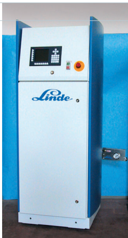
Fig. 4. The high-pressure metering unit compresses the blowing agent to pressures of up to 500 bar
