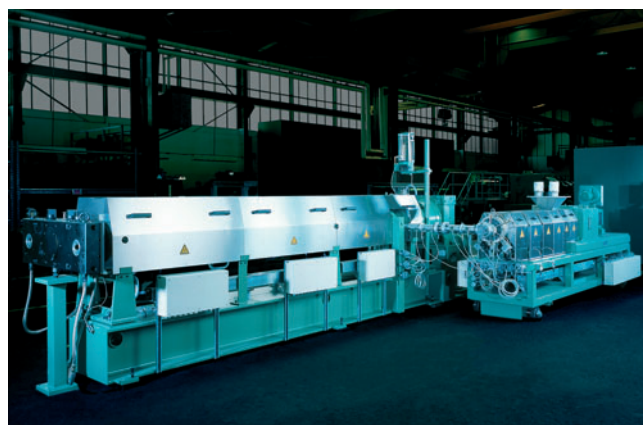
Fig. 1. Foam extrusion machine in tandem arrangement with twin-screw extruder and single-screw extruder (photo: Berstorff)
